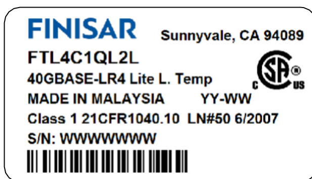
Figure 3 – FTL4C1QL2L label (not to scale)
