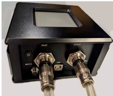
Figure 13. Water Hoses With Step-down Fittings
