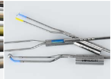
Ultra-short pulsed laser black marking of stainless steel
