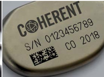
Ultra-short pulsed laser black marking of titanium
