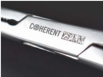
Ultra-short pulsed laser black marking of stainless steel
