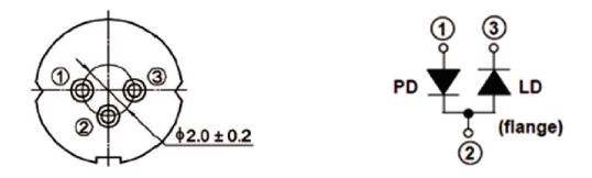
1. PD Anode; 2. LD Anode/PD Cathode; 3. LD Cathode
