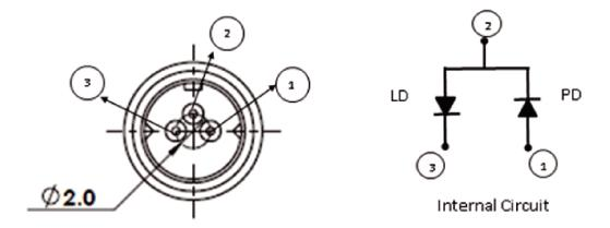
1. PD Anode; 2. COM (LD Anode, PD Cathode); 3. LD Cathode
