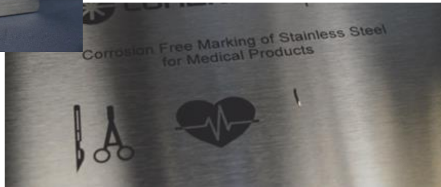
Nanosecond laser marking after corrosion test (72h in 50°C warm 5% NaCl salt-water spray test)
