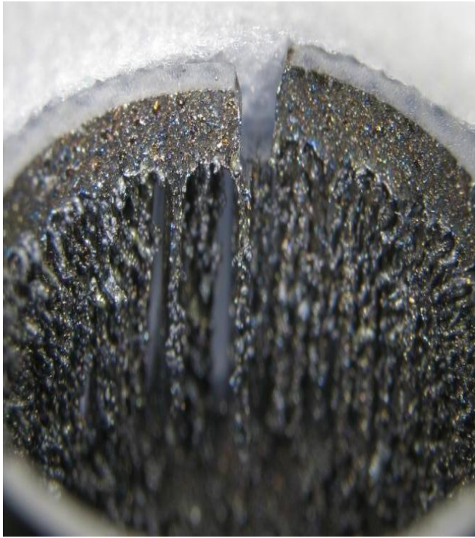
dry cutting, PowerLine FL 200 Required cleaning: mechanical deburring
