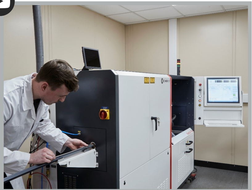
Figure 1. The side access of the StarCut Tube enables Micrometric to easily process long tubes. Image courtesy of Micrometric.
