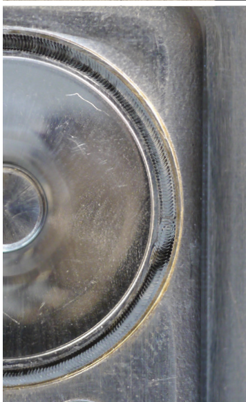
Battery cell: CID (Al/Al) welding
