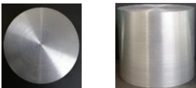
Figure 2. Aluminum-scandium alloy billet
