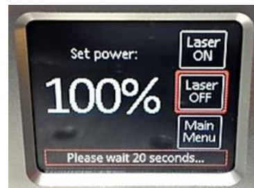
LCD Control Panel, indicating all interlocks are satisfied, laser “ON” controls have been activated, and laser emission will occur after the 20 second delay has counted out.
