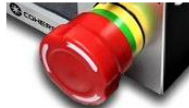
Green ‘color-band’ exposed on E-Stop indicating emission can occur when all laser controls are activated and all other interlocks are satisfied.
