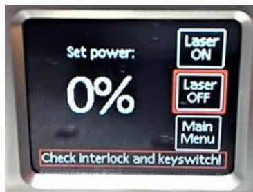
LCD Control Panel, indicating status of Remote Interlock I/O, and/or Keyswitch is disabled. Thus, no laser emission can occur until those controls are satisfied.
