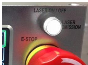
Laser On/Off Button / Emission Indicator-LED, lit, indicating all interlocks are satisfied, laser “ON” controls have been activated and laser emission is occurring.
