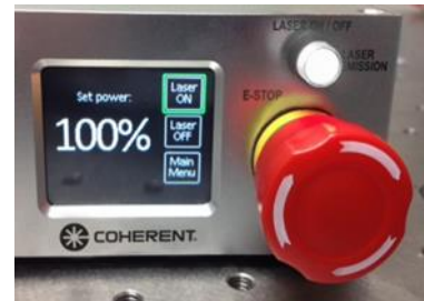
All Front Panel indicators active, indicating all interlocks are satisfied, laser “ON” controls have been activated and laser emission is occurring.
