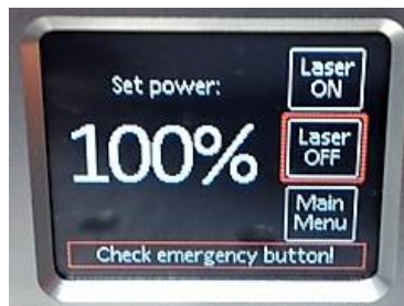
LCD Control Panel indicating both Remote Interlock I/O and Keyswitch are satisfied, but the E-Stop is not. Thus, no laser emission can occur until that control is also satisfied.
