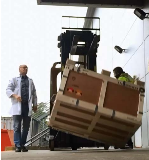
Figure 5. A Chameleon Discovery laser is dropped 2m from a forklift during the exhaustive HALT design phase
