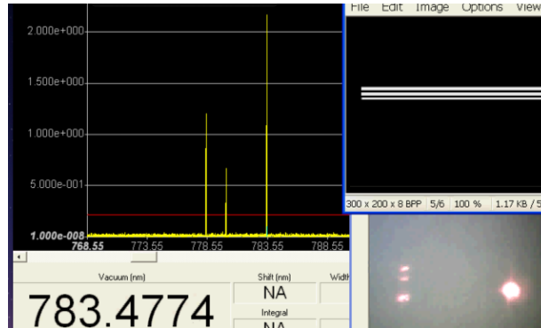
Fig. 6. Multi-line operation while maintaining single mode for each line
