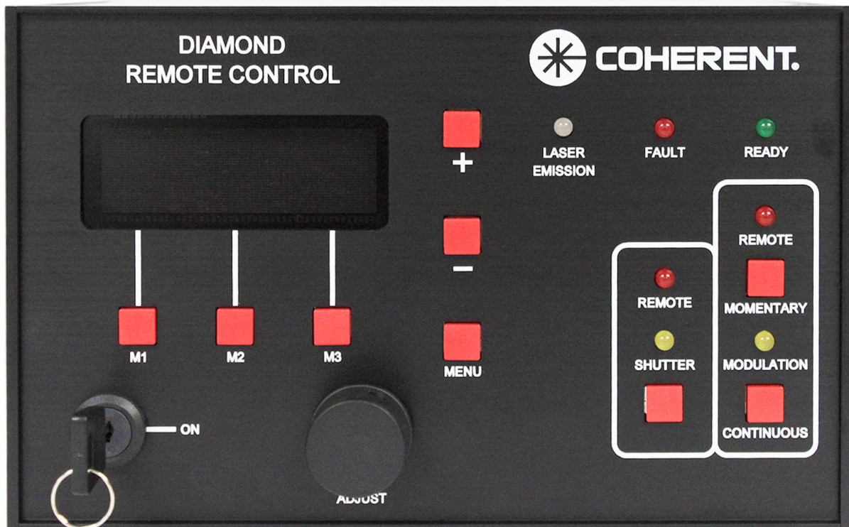
Figure 5-8. Diamond Remote Control
