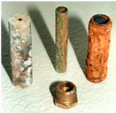
Untreated Water Circuit
