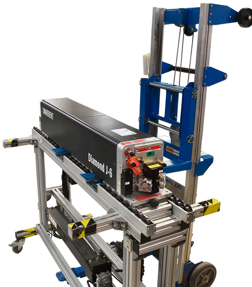
Figure 4-9. Lifting the Laser (Continued)
